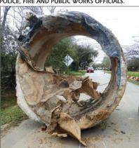
THIS IS THE SECTION OF OLD PIPE THAT FAILED AND FLOODED THE STREETS.
