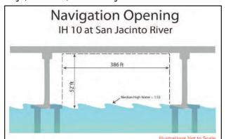
The new roadway will be 30' higher than existing. The navigational opening for boats is increased in height and width to reduce impacts to the bridge structure and bumpers.
