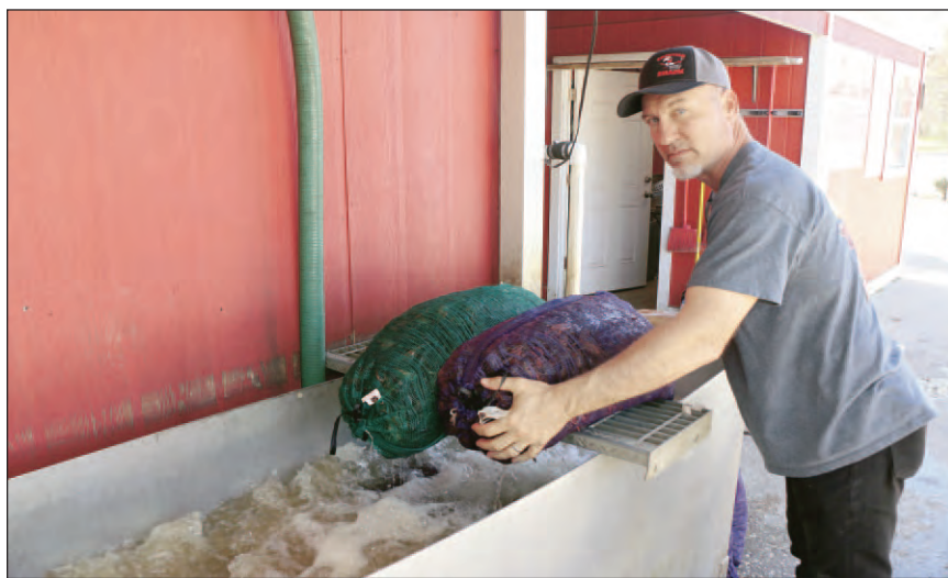
Dan Meaux removes two bags from the aerator tank, a sort of jacuzzi for the crawfish that stays in the tub up to an hour to remove any remaining dirt and sand from the mudbugs before they head to the boil room. Only about 10 percent of restaurants across Houston have the equipment which makes them extremely clean before boiling.
