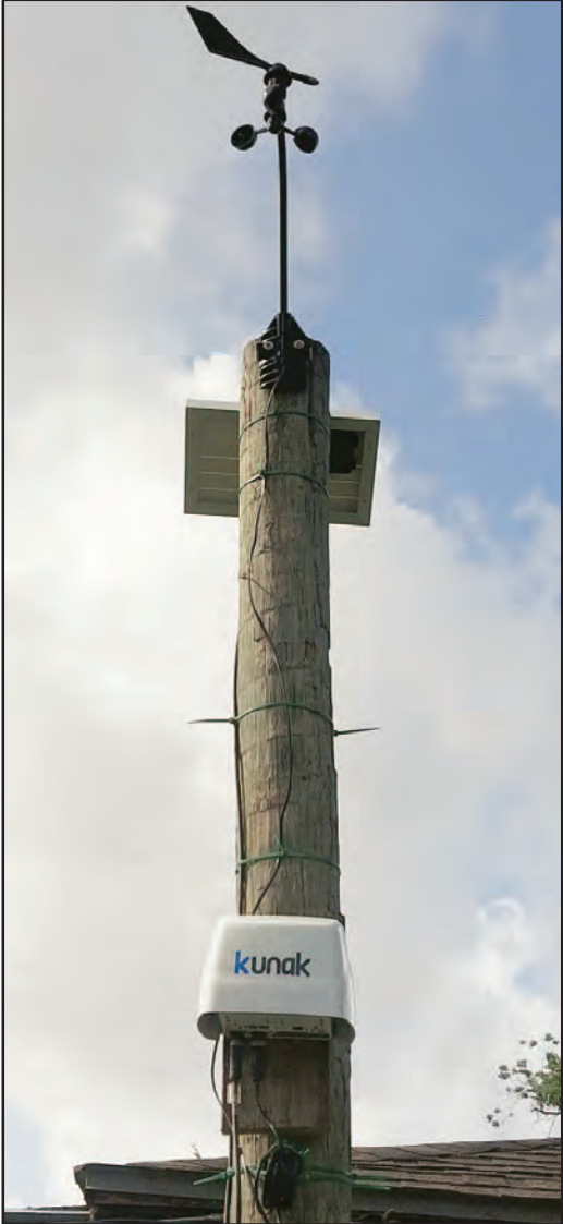
A Kunak air monitor measures air quality outside a Channelview home. The monitor was the first of the new monitors being installed in Channelview, and is capable of detecting particulate matter, nitrogen dioxide, ozone pollution, carbon monoxide, and volatile organic compounds. Photo provided by Carolyn Stone.
